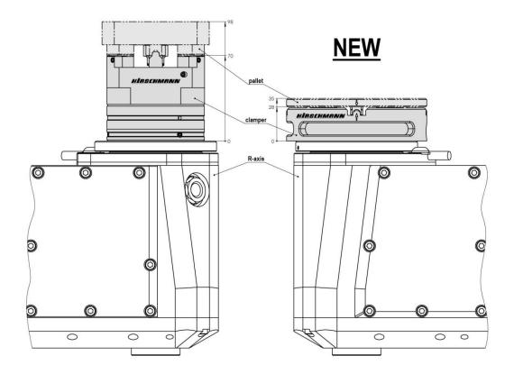
Difference in height is evident: clamping system  $\mu$ -PrisFix-Flat (on the right) is considerably flatter than previous reference systems. This raises efficieny of machining processes. Picture: HIRSCHMANN GMBH
